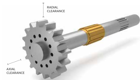
FIGURE 29 - RADIAL AND AXIAL CLEARANCE ON A POLE WHEEL.
